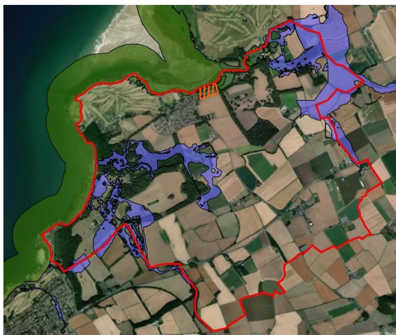
Map showing SEPA Medium Likelihood of Coastal (green) and River (purple) Flooding with proposed area for flood mitigation (orange)
